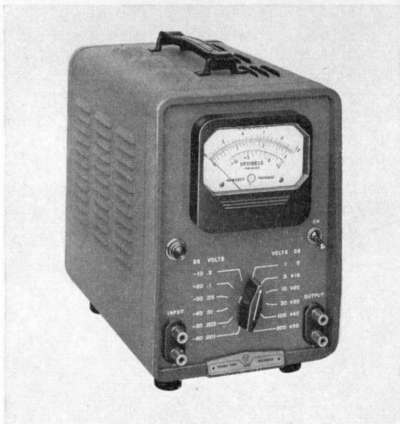
Fig. 1. New -hp- Model 400D measures voltages from 10 cps to 4 megacycles down to levels as low as 100 microvolts. Output terminals permit use as wide-band amplifier.
